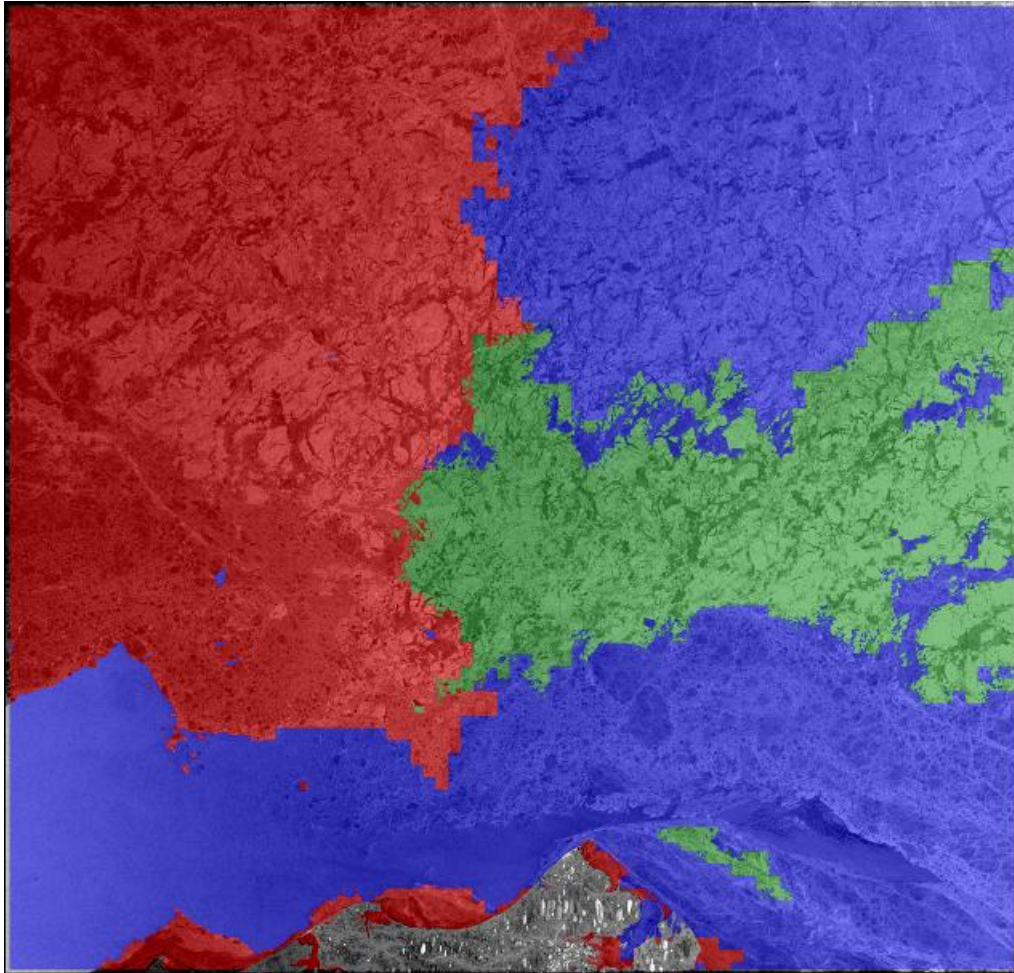
Figure 6.8: HH,HV Glocal result for Figure 6.3 for polygon size 128. The strong illumination in HH throws off the algorithm. Blocky artefacts are introduced.
